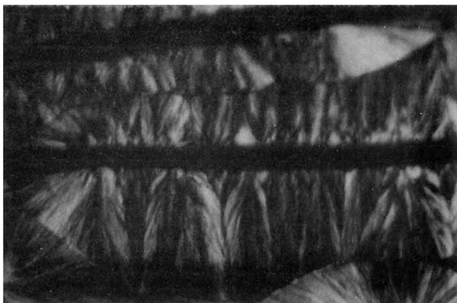
Fig. 7. Polarized optical micrograph of PB-1 crystal grown at 90°C from the melt (a) on a glass plate and (b) in contact with PP fibers.
